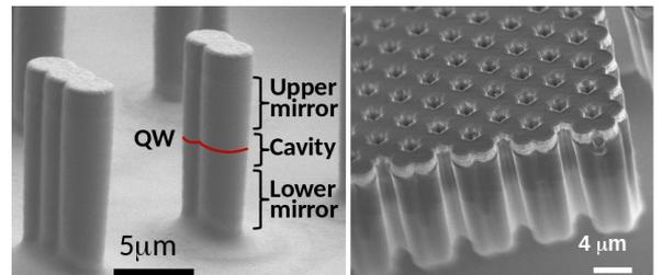
FIG. 1: Left: set of two and three deeply etched coupled micropillars. Right: honeycomb lattice of micropillars.
